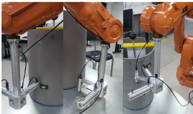
Figure 13: Automatic measurements on the last layer performed by the robotic system.
