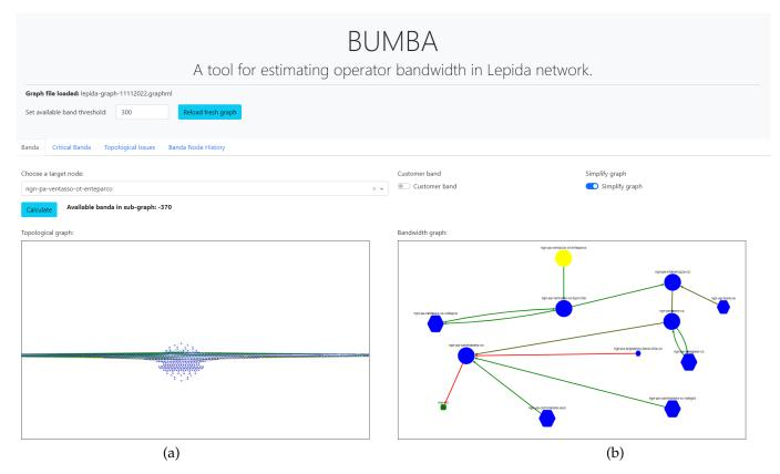
Figure 7: The *Banda* tab is where the residual band is calculated for a single, selected target node. When the filtered graph is too large, as depicted in the left graph plot window (7a), by enabling the *Simplify graph* widget the graph is reduced and simplified while still retaining the information about the selected target residual band (7b).
