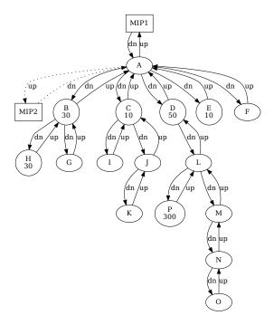
Figure 1: Network graph from which has been extracted the node L subgraph. END POINTs are depicted as a rectangular box, while other nodes are elliptic boxes. When present, the number inside a node box represents the allocated, total operator bandwidth.
