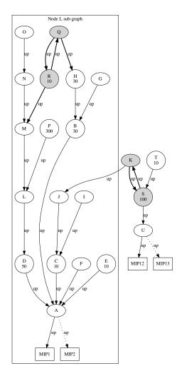
Figure 2: Prototypical, but more realistic representation of node L subgraph. The gray filled shapes of nodes Q, R, K and S represent a *chain* structure where all edges are tagged as *up-links*. Two distinct pairs of MIP nodes are shown and are linked to distinct (PAL) nodes (i.e., A and U). The box on the left encloses node L sub-graph (LG) after the final filtering. Due to consecutive filtering processes, only up-links are left as they are exploited by the calculation algorithms.
