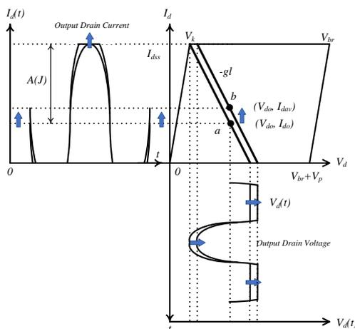
Figure 1: Principles of the load-line analysis. Drain current  $I_d(t)$  and drain voltage  $V_d(t)$  swing on the load-line having a resistive slope of  $-g_l$  within the area surrounded by  $V_k$  (Knee voltage),  $V_{br}$  (breakdown voltage),  $V_{br}+V_p$  ( $V_p$  is a pinchoff voltage) and zero. Point  $a$  is an initial bias condition ( $V_{do}$ ,  $I_{do}$ ). Point  $b$  is a final bias condition ( $V_{do}$ ,  $I_{dav}$ ).
