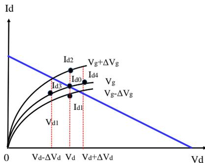
Figure 4: Nonlinear circuit elements of gm, R<sub>ds</sub>, C<sub>gs</sub> and C<sub>dg</sub> obtained from I-V curves as a function of V<sub>g</sub> and V<sub>d</sub>
