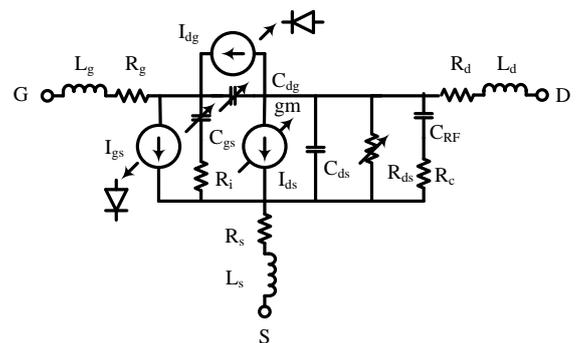
Figure 3: Large-signal GaN HEMT model.  $L_g$ ,  $R_g$ ,  $L_s$ ,  $R_s$ ,  $L_d$  and  $R_d$  are an extrinsic element, which are linear and thus keep a constant value. On the other hand,  $R_i$ ,  $C_{ds}$ ,  $C_{RF}$  and  $R_c$  are an intrinsic element, which are also linear and thus keep a fixed value.  $R_{ds}$  is used to represent DC characteristics. Therefore, RF characteristics are represented by  $1/(1/R_{ds} + 1/R_c)$  for a large value of  $C_{RF}$ .
