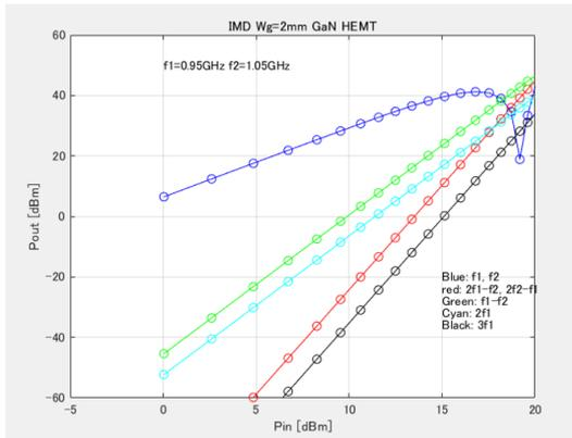
Figure 10: The 1<sup>st</sup>-, 2<sup>nd</sup>- and 3<sup>rd</sup>-order products. Red curve is the 3<sup>rd</sup>-order product ( $2\omega_1-\omega_2$  or  $2\omega_2-\omega_1$ ), which appear in close to carrier frequencies of  $\omega_1$  and  $\omega_2$ .
