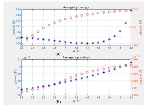
Figure 5: Calculated gm<sub>ave</sub>, g<sub>dsave</sub>, C<sub>gsave</sub> and C<sub>dgave</sub>. Under class-B operation with a tuned load, I<sub>d</sub>(t) moves partly on the load-line with zero gm. Thus, the averaged gm sometimes decreases with A(J). However, the bias point moves upward and the averaged current also increases with A(J). Then gm drastically increases.
