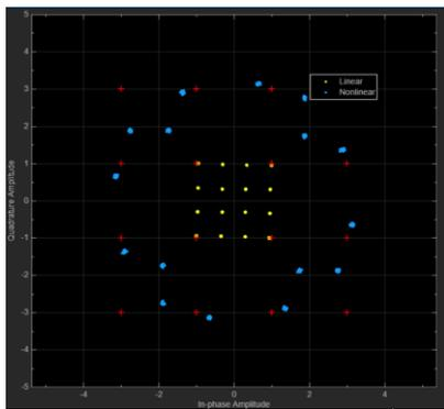
Figure 14: Constellation diagram of 16-QAM modulated signal. Red and blue dots are ideal and distorted signals at  $P_{in}$  of 20dBm. Red and yellow dots are ideal and distorted signals at  $P_{in}$  of 5dBm. It can be clearly shown that the constellation is seriously distorted at  $P_{in}$  of 20dBm (blue dots).
