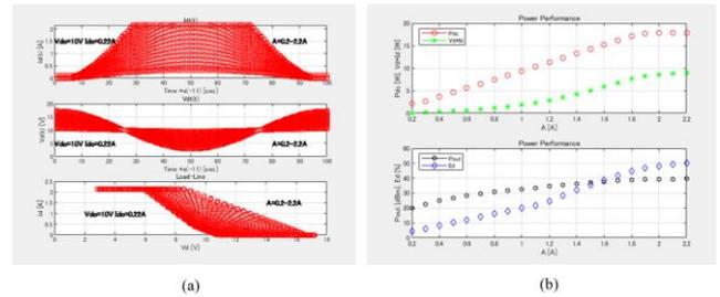
Figure 2: (a) Calculated  $I_d(t)$ ,  $V_d(t)$  and dynamic load-line. (b) Calculated  $P_{out}$ ,  $\eta_d$ ,  $P_{dc}$  and  $V_d \times I_d$  for GaN HEMT devices with  $V_k$  of 2V,  $V_{br}$  of 100V,  $V_p$  of -2V and  $I_{dss}$  of 2.14A
