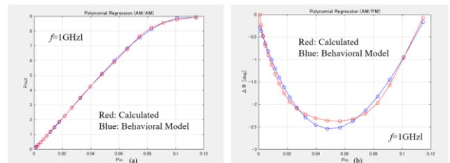
Figure 9: Calculated AM-AM and AM-PM performances combined with behavioral modeling. (a) AM-AM performance at 1GHz. (b) AM-PM performance at 1GHz.  $P_{\text{out}}$  and  $P_{\text{in}}$  are antilog number.  $\Delta\phi$  is represented as degree
