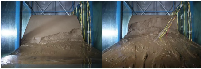
Figure 15: laboratory slope erosion during rainfall
