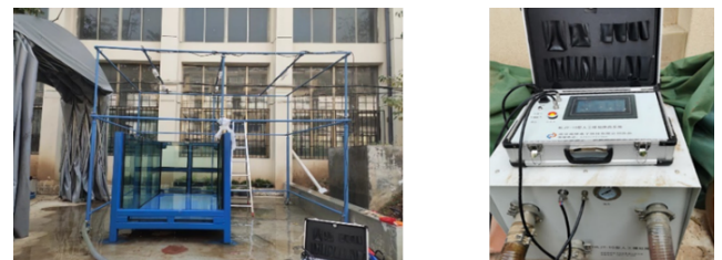
Figure 2: Artificial simulated rainfall system
