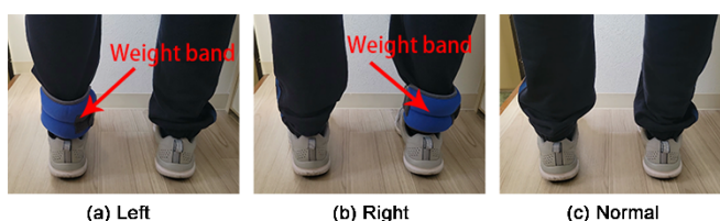
Figure 1: Experimental conditions of gait measurement including (a) weight band attached to the left ankle, (b) weight band attached to the right ankle, and (c) normal gait without additional weight.
