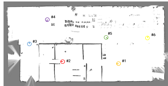
Figure 16: Positions selected on the map for the global localization experiment.
