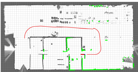
Figure 22: Real-time trajectory of the robot shown on the map in the actual workshop environment.
