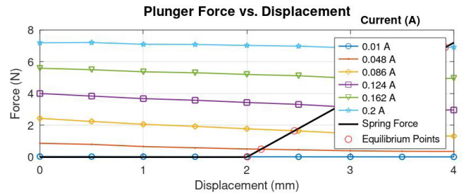
Figure 27: Force vs Displacement characteristics of the Proportional Solenoid and the restraining spring (2 mm offset)
