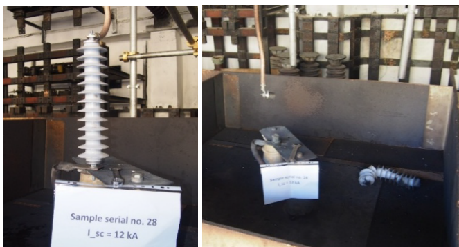
Figure 16: Aspect of the surge arrester before and after short-circuit test at 12 kA
