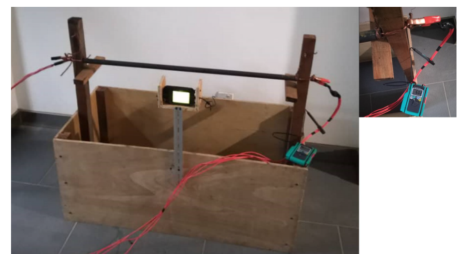
Figure 7: The setup used to determine the heat generated on the pipe
