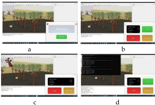
Figure 16: a. The robot in the field with the interface of the control panel, b. The robot moving on the field, c. The robot reached a palm and stop using the LiDAR. D. The robot use the camera, capture images that sent to the YOLO Module
